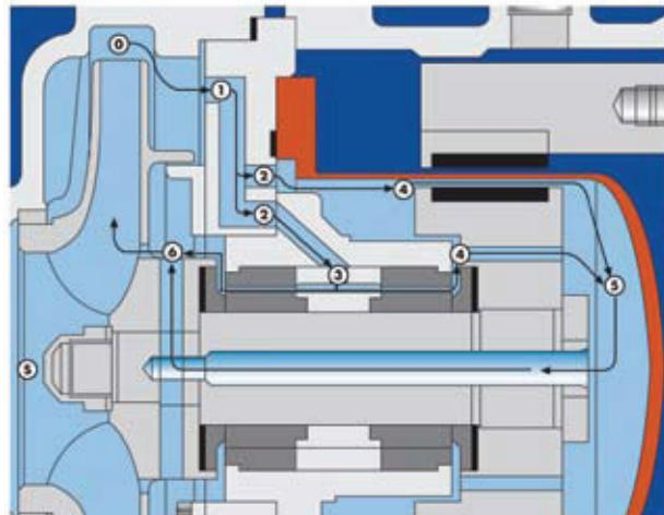
Figure 2. Lubricating and cooling circuit for boiling liquids.
