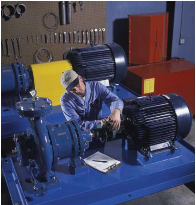
Mag-drive pumps now exceed driving power of 500-hp, flow rates of 15,000-gpm, delivery heads of 3,000-ft tdh, system pressures of 5,800-psi, operating temperatures of 840-deg F without cooling, and viscosities of 3,000-cPs.
