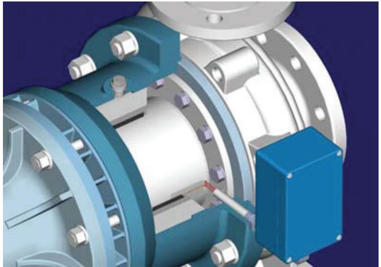
**Figure 3. TPS system to monitor isolation shell temperature.**
