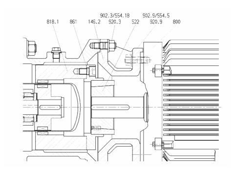
When using a US-NEMA motor by way of driving motor (part no. 800), the outer magnet carrier hub (part no. 861) will be secured on the motor shaft by means of a Taper-Lock fastening element (part no. 522). The two-part Taper-Lock fastening element comprises the inner fastening bush and the outer reduction sleeve.
